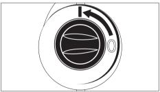
Turn on the pressure washer (I). **NOTE**: This unit is equipped with a pressure switch. The motor only starts up when the trigger on the gun is pulled.
