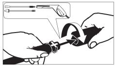
**Step 2**Insert the variopower nozzle or the rotary nozzle into the trigger gun. Press in against the spring tension and twist into the locked position.
